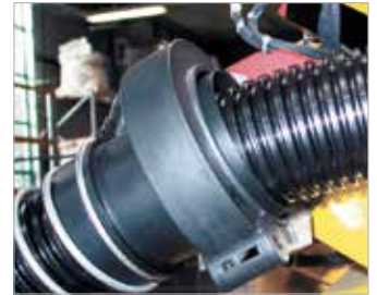
■ Tube clamp with gliding bush
