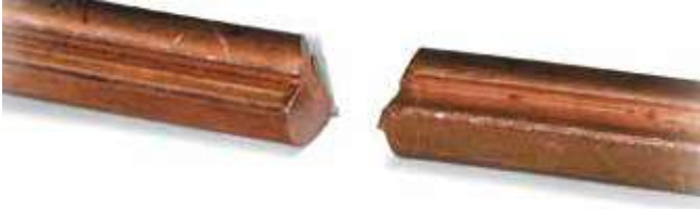
Contact wire cut with a traditional cutter
