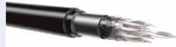
Same as lead protection against aromatic hydrocarbons and active chemicals. This design combining aluminium tape and high density polyethylene HDPE sheath with a covering of polyamide PA (Nylon), represents an excellent barrier against penetrating chemicals and can be used as an alternative to lead sheath. Advantage: lighter, smaller diameter.
