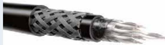
Lightweight armour to withstand tensile loads; permits the smallest bending radii of all armour designs; used mainly for small cable diameters; a coverage of at least 80 % and a wire diameter of 0.3 mm are recommended to achieve sufficient mechanical protection.
