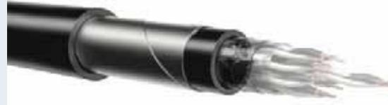
Double layer, lapped steel tapes, 100 % covering of the cable assembly. Good protection against pressure, impact loads and rodents, not suitable for tensile loads. Best inductive protection of all armours listed.
