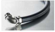
Liquid-tight LTS conduits, combined with LTS fittings, provide IP68 and IP69k ingress protection. LTS conduits deliver exceptionally high compression, tensile and impact strength. The smooth outer cover is resistant to liquid fuel, oils and grease.
