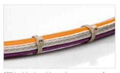
PEEK cable ties withstand temperatures from -55° C up to +240° C. They are resistant to gamma radiation and chemicals - even acids. The tie is outside-serrated and the head geometry optimised to minimise the risk of any damage to cable insulation.
