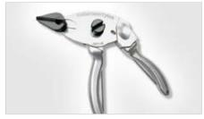
The HDT16 application tool is designed for installing heavy duty stainless steel cable ties. The two-way nose piece can be adjusted so that MBT, MLT and AMT cable ties with a strap width of up to 16 mm can be easily applied. The integrated cutting mechanism delivers a flush, safe cut every time.
